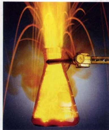
The reaction between sodium and bromine
